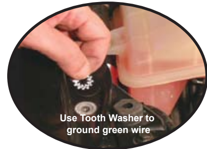
Tooth Washer must penetrate paint for clean contact with metal
